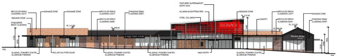
Supermarket/Retail East Elevation Scale 1 : 200
