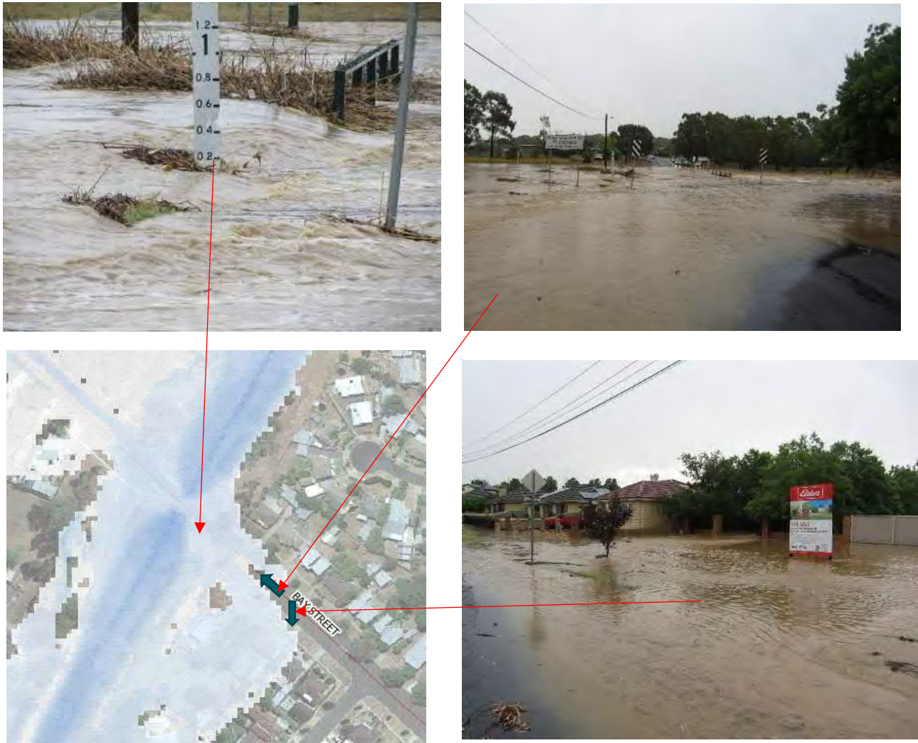
Figure 2-4 January 2015 Flooding at Bay Street Bridge imagery vs. model result
