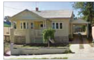
New car parking structures that are smaller in scale than the dwelling, recessed, set under the eaves and have a simple gable roof.
