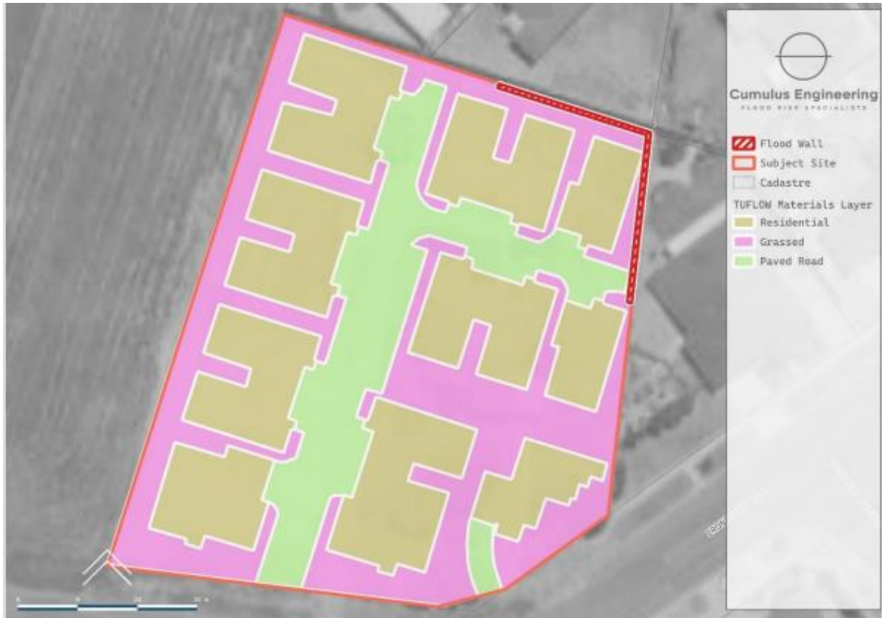
Figure 9. Excerpt from Flood Assessment showing developed conditions of the site and the location of the flood wall.
