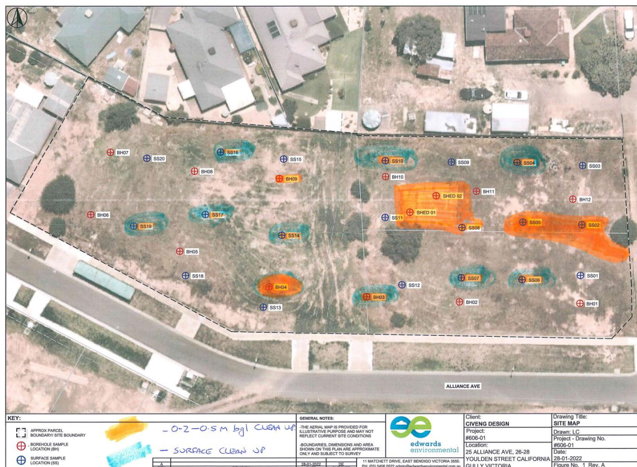
Figure 13: Plan showing boreholes and where clean up of the site is required (source: Preliminary Environmental Site Assessment, 25 Alliance Avenue & 26-28 Youlden Street California Gully, prepared by Auburn Consulting Group)
