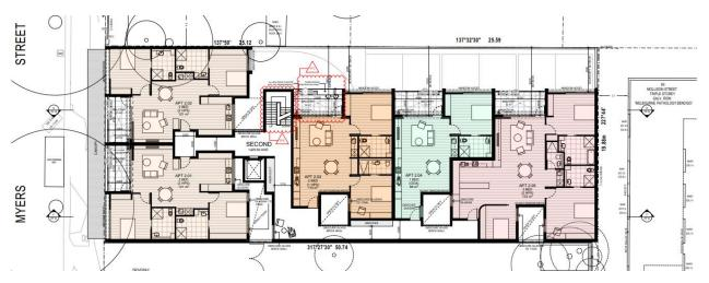
Figure 6: Proposed Second Floor Plan
